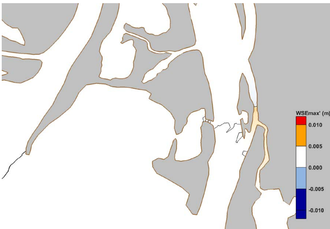
Figure 59. Predicted Change in Maximum Water Elevation (WSEmax') from Case 002 to Case 302
