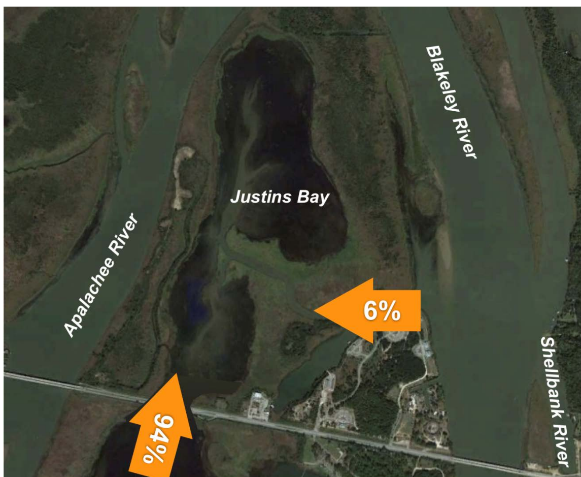
Figure 54. Distribution and Direction of Tidal Exchange Volumes in Justins Bay for Case 202, Expressed as Percentages of the Total Volume of Water Exchanged
