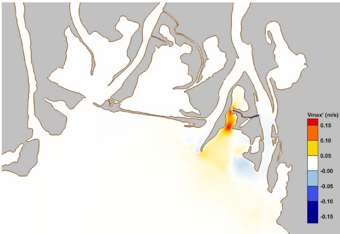
Figure 51. Predicted Change in Maximum Depth-averaged Velocity ( V_{max}' ) Between Case 202 and Case 002
