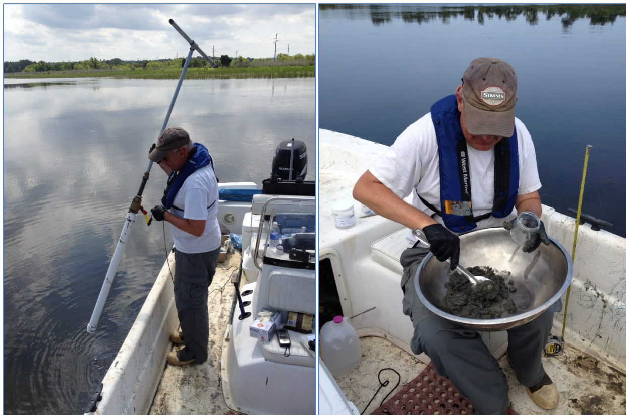
Figure 3. Pushcore Sediment Sampling and Processing in Justins Bay
