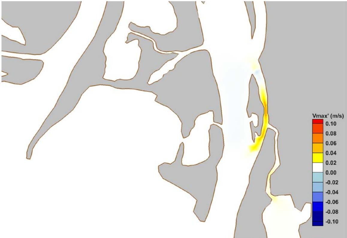
Figure 60. Predicted Change in Maximum Water Velocity ( V_{max}' ) from Case 002 to Case 302
