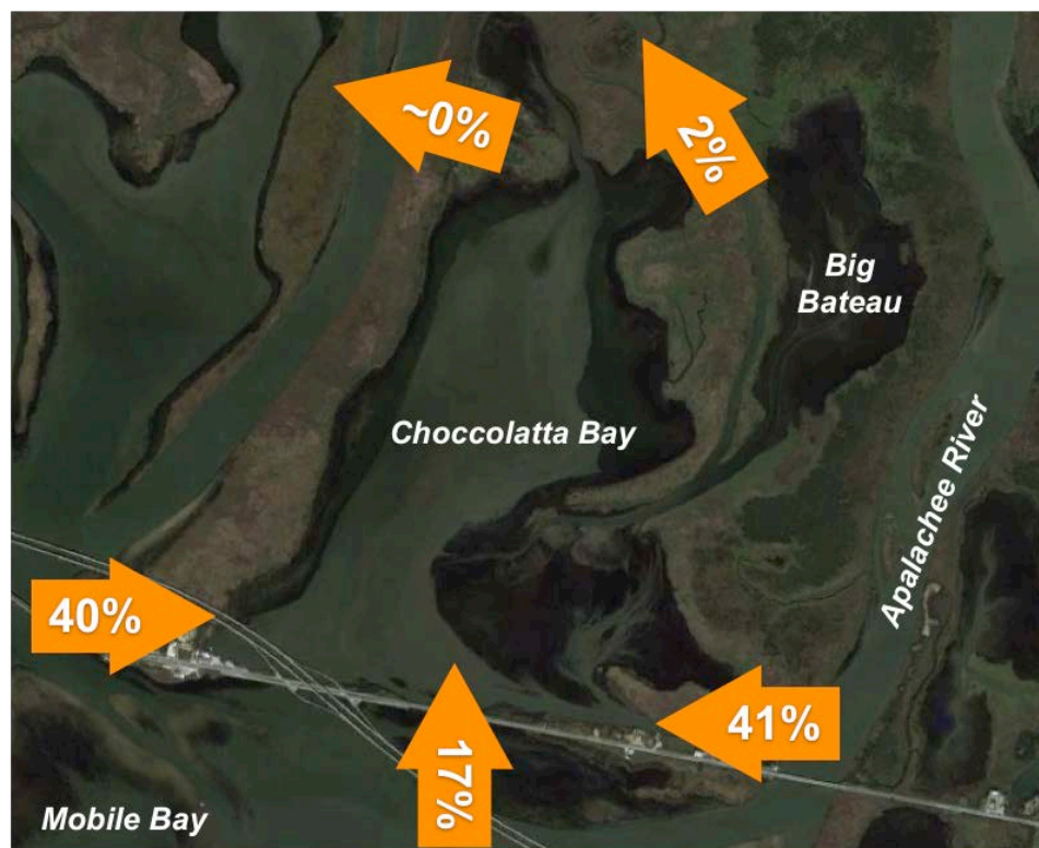
Figure 31. Distribution and Direction of Tidal Exchange Volumes for Choccolatta Bay under Existing Conditions (Case 002). Values are Shown as Percentages of the Total Volume of Water Exchanged
