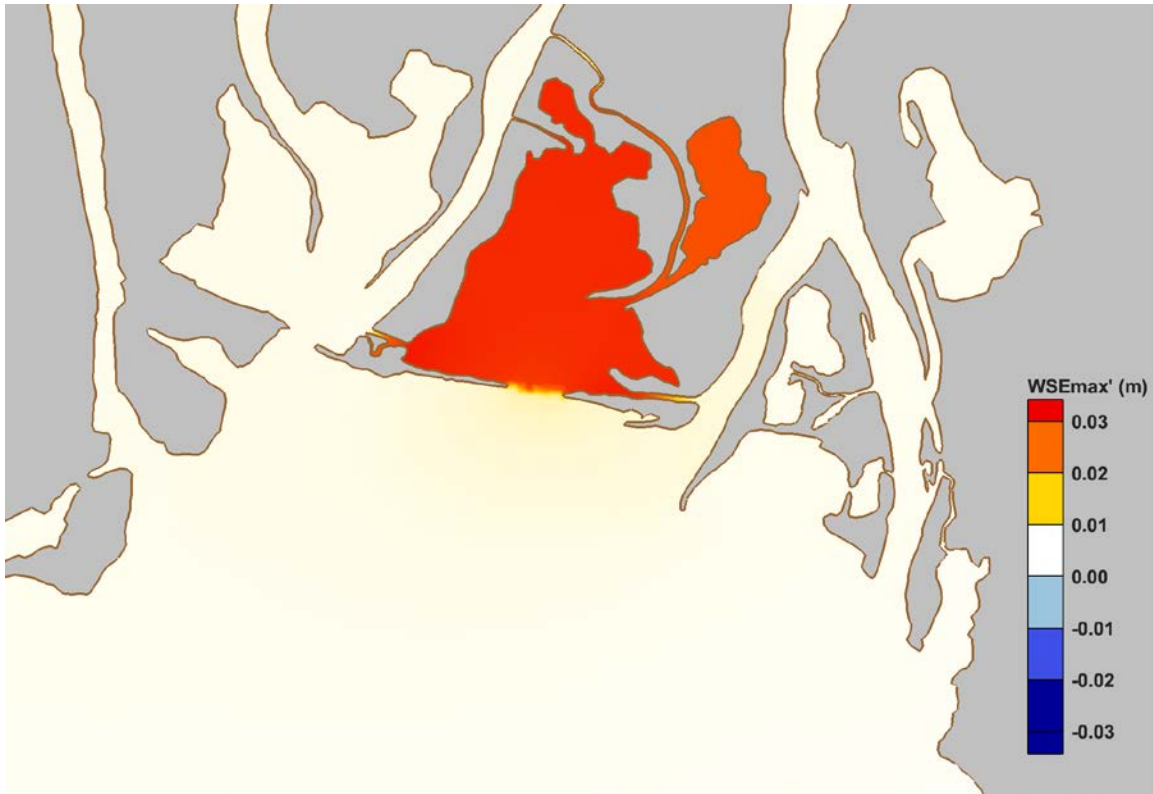
Figure 36. Change in Maximum Water Levels (WSEmax') for Case 102, Shown in Meters. Positive Values Show Increases Relative to Existing Conditions and Negative Values Show Decreases
