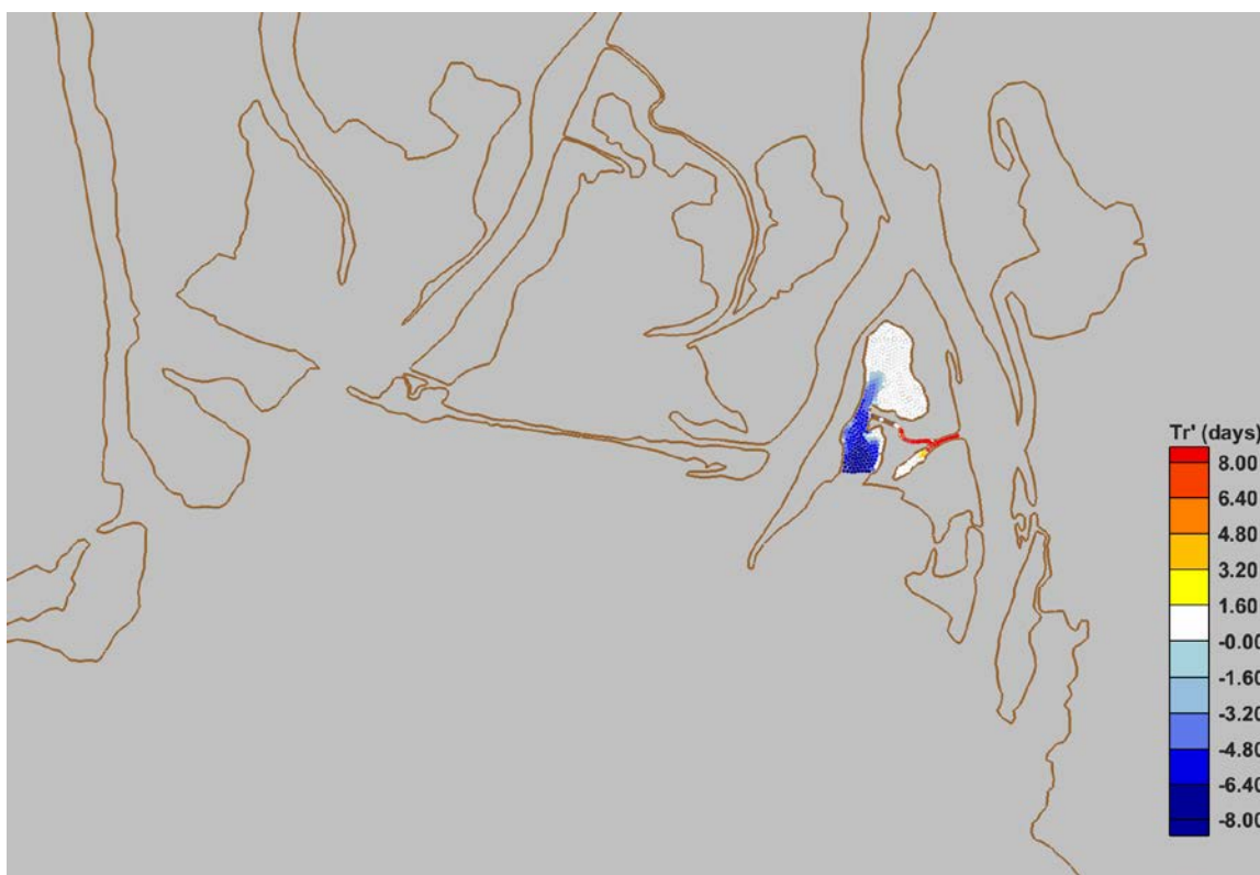
Figure 58. Predicted Change in Residence Time ( Tr' ) from Case 002 to Case 202 as a Function of Particle Initial Position
